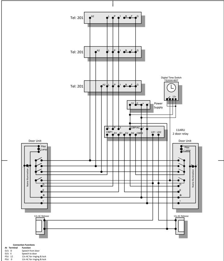
12v AC for ringing & lock 12v AC for ringing & lock 12v DC for speech & lamps 12v DC for speech & lamps PSU 0 PSU + SC FEL A2 TEL A1 TEL L TEL P Ringer Warble Ringer buzzer (if fitted) Speech from door Speech to door TEL 1 B Lock button Common for ringers TEL TEL Common for speech TEL G Common for buttons 11ARU CBP1-2 Door button feeds 11ARU D1-2 11ARU E1-2 Speech from Panels Speech to Panels
