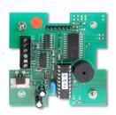
The PN4PM is designed to fit as an integral part of an Entryphone entrance panel. The reader will be fitted into the panel at manufacture.
